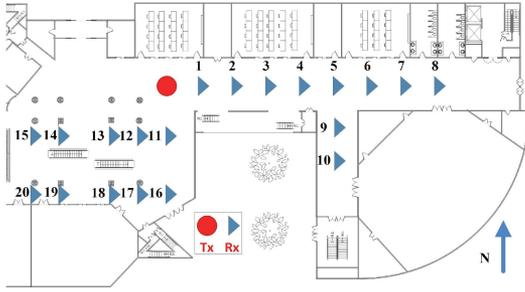
Fig. 1. Measurement map, pos 1–8, 11, and 16 have LoS conditions, pos 9, 10, and 17–20 have NLoS conditions, and pos 12–15 have OLoS conditions.
