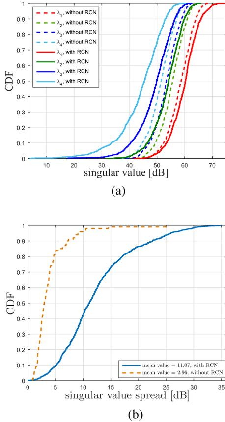
Fig. 4. Comparisons of singular value distributions using the IMT-2020 channel model with and without the RCN feature. (a) Largest four singular values. (b) Singular value spread.
