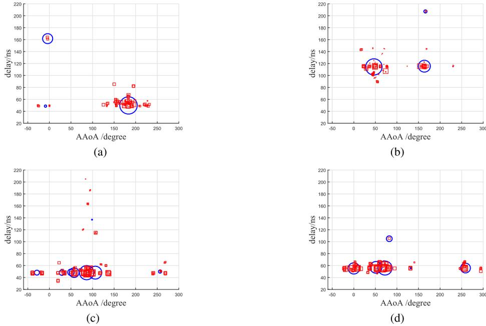
Fig. 2. Four examples of the delay-AAoA profiles of clusters ( $90^\circ$  faces the north direction) in Cartesian coordinates. Each blue circle represents the position of a cluster, while each red square represents the position of an MPC. The size shows its power in dB. (a) pos 3 (LoS). (b) pos 10 (NLoS). (c) pos 11 (OLoS). (d) pos 17 (NLoS).
