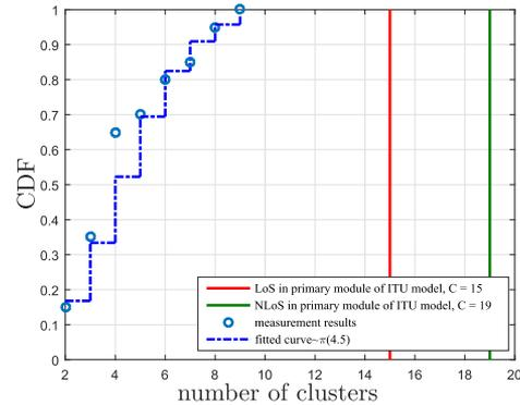
Fig. 3. CDFs of the number of clusters in the measurements, Poisson-based simulation, and listed in the primary module of the IMT-2020 model.
