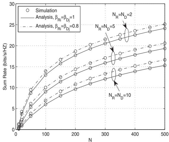
Fig. 4. The achievable sum rate versus  $N$  with different number of interferers ( $K = 5$ ,  $\rho_1 = \rho_2 = 0$  dB,  $\rho_{Ri} = \rho_{Dj} = 0$  dB,  $\forall i, j$ ).
