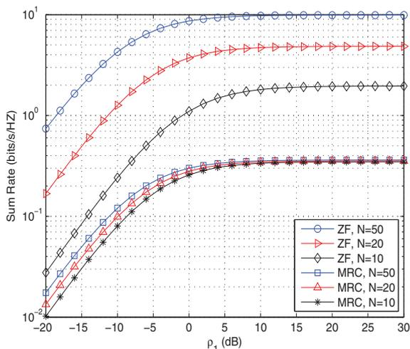
Fig. 5. Comparison of simulation results for ZF and MRC scheme ( $K = 5$ ,  $N_R = N_D = 2$ ,  $\rho_2 = 0$  dB,  $\rho_{Ri} = \rho_{Dj} = 0$  dB,  $\beta_{Ri} = \beta_{Dj} = 1$ ,  $\forall i, j$ ).
