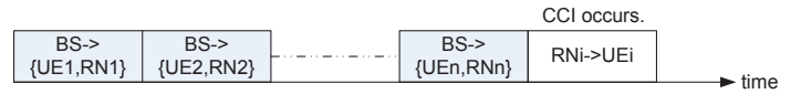
Fig. 2. Resource allocation for the cooperative transmission. The last time slot with the slashed background is the relay-transmit phase. RNs transmit to its assigned UE simultaneously in this time slot.
