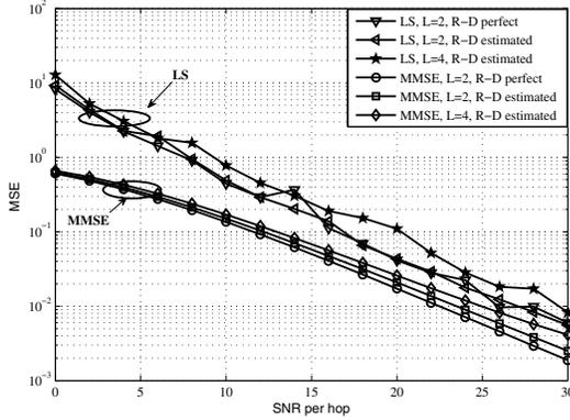
Fig. 3. Channel estimation MSE of S-R link.
