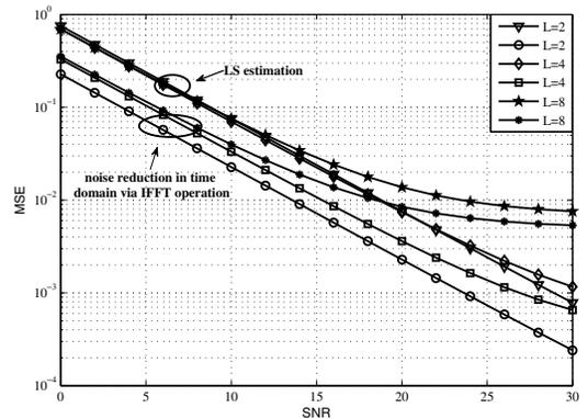
Fig. 2. Channel estimation MSE of R-D link.
