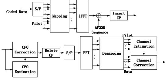
Figure 1. Block diagram of the proposed APSSB OFDMA
